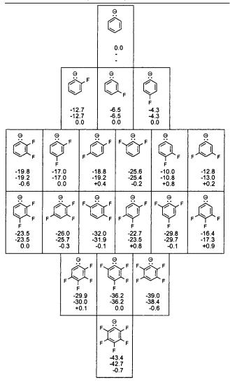
[a] All numbers in kcal mol<sup>-1</sup>. [b] B3 LYP/aug-cc-pVTZ//B3 LYP/cc-pVTZ. [c] Each fluorine atom in *ortho*, *meta*, and *para* to the carbanion center is assumed to lower the proton affinity by 12.7, 6.5, and 4.3 kcal mol<sup>-1</sup>, respectively.
